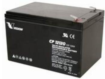
The rechargeable batteries are lead-lead dioxide systems. The dilute sulfuric acid electrolyte is absorbed by separators and plates and thus immobilized. Should the battery be accidentally overcharged producing hydrogen and oxygen, special one-way valves allow the gases to escape thus avoiding excessive pressure build-up. Otherwise, the battery is completely sealed and is, therefore, maintenance-free, leak proof and usable in any position.
